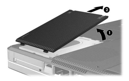
4. To remove the hard drive, pull upward on the hard drive tab **1** to release the hard drive, and then lift the hard drive **2** out of the hard drive bay.
